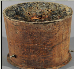
Directionally Focused Fragmentation Charge -DFFC
