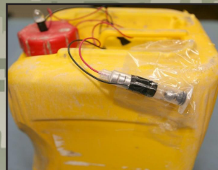
YPOC w/ Booby Trap Anti-Tilt Switch -Syringe
